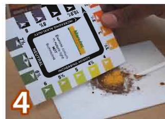
4 The white barium powder changes to a different colour, compare the new colour against closest colour on the colour chart to obtain a pH reading.
