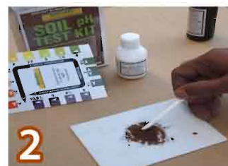
2 Then mix the indicator liquid with the soil sample to make a thick paste.
