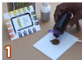
1 Take a small soil sample on the white mixing plate and add a few drops of indicator dye.
