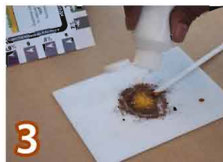
3 Sprinkle white Barium powder from the puffer bottle on to the top of moist soil paste.
